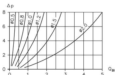
Figure 7:  $Q_{BI}$  flow rate (lpm);  $\Delta p$  flow resistance (bar) with responding LB valve
