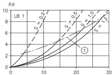
Figure 2:  $Q_{LB}$  flow rate (lpm);  $\Delta p$  flow resistance (bar)
