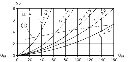
Figure 5:  $Q_{LB}$  flow rate (lpm);  $\Delta p$  flow resistance (bar)
