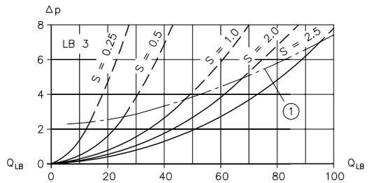
Figure 3:  $Q_{LB}$  flow rate (lpm);  $\Delta p$  flow resistance (bar)
