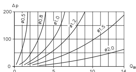
Figure 8:  $Q_{BI}$  flow rate (lpm);  $\Delta p$  flow resistance (bar)  $\approx$  load pressure
