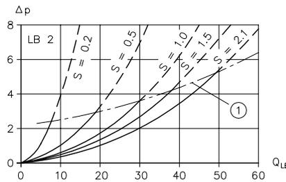
Figure 4:  $Q_{LB}$  flow rate (lpm);  $\Delta p$  flow resistance (bar)
