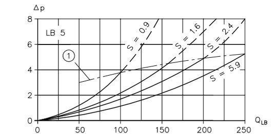
Figure 6:  $Q_{LB}$  flow rate (lpm);  $\Delta p$  flow resistance (bar)
