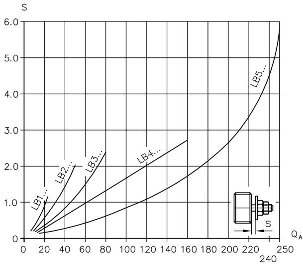
Figure 9:  $Q_A$  flow rate (lpm);  $S$  gap width (mm)
