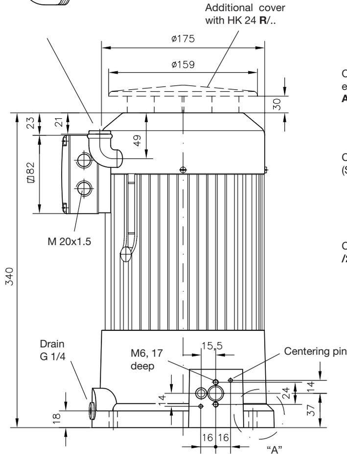
Orientation of the upper part of the pump with terminal enclosure
