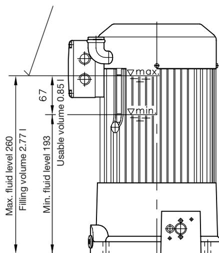
The specific usable filling volume is 0.12 l per 10 mm of fluid level drop. The motor outline (winding overhang) is no longer oil immersed if the fluid level drops below the min. marking. Any further drop will result in no considerable volume gain as the bottom interior is occupied by functional parts.
