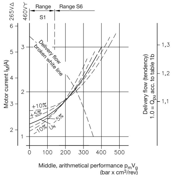
The product of  $pV_g$  (bar · cm<sup>3</sup>/rev) is laid off as abscissa in these curves. This makes a rough consideration possible for the current and the delivery flow to be expected, which is sufficient under most conditions.
